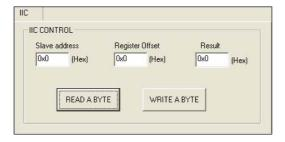
When the application is executed, you can read or write a byte of data through I<sup>2</sup>C devices. All data must be read or written in hexadecimal system.
