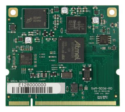
This document describes EMAC's SoM-A5D36 System on Modules (SoMs). The SoM-A5D36 is a System on Module, designed to be compatible with EMAC's 200-pin SODIMM form factor. This module is built around the Atmel ATSAMA5D3x ARM based microcontrollers, which provide several of its key features.
