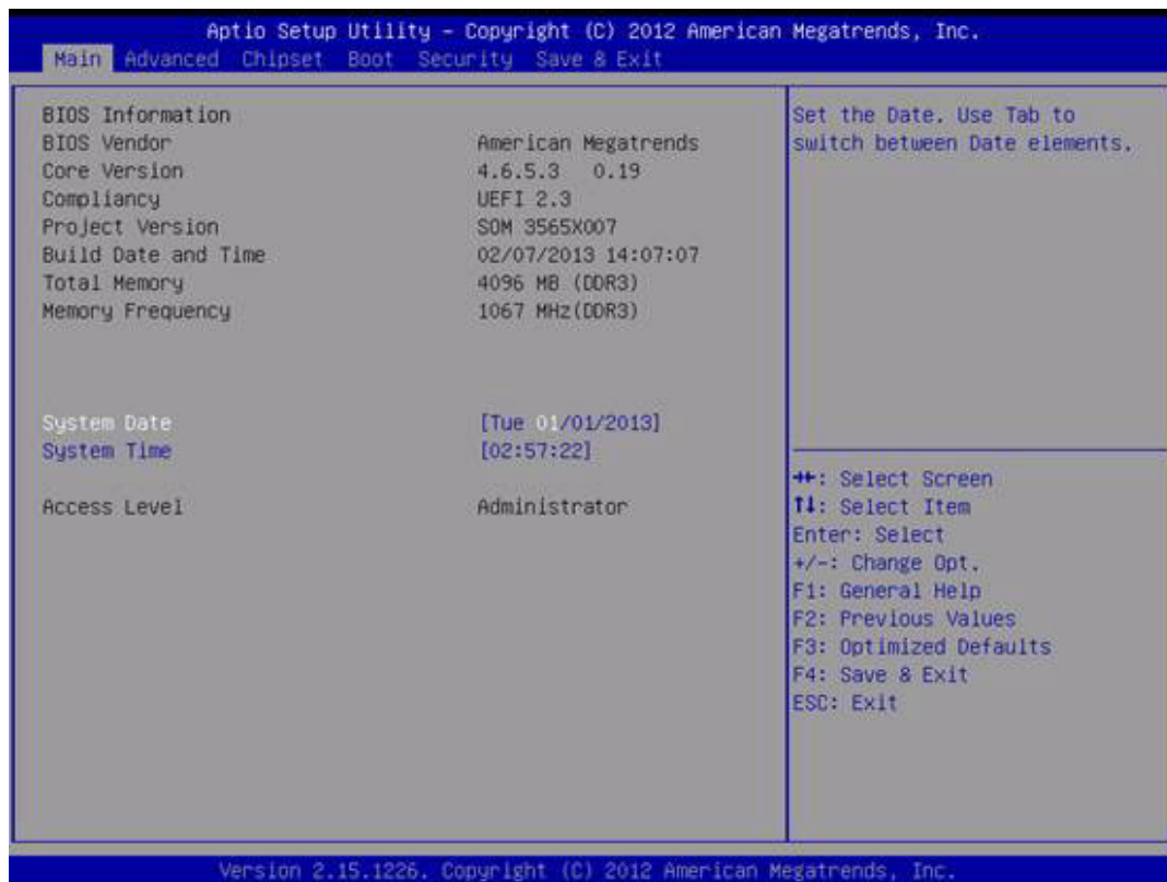
Figure 3.1 BIOS Setup Utility Main Screen
