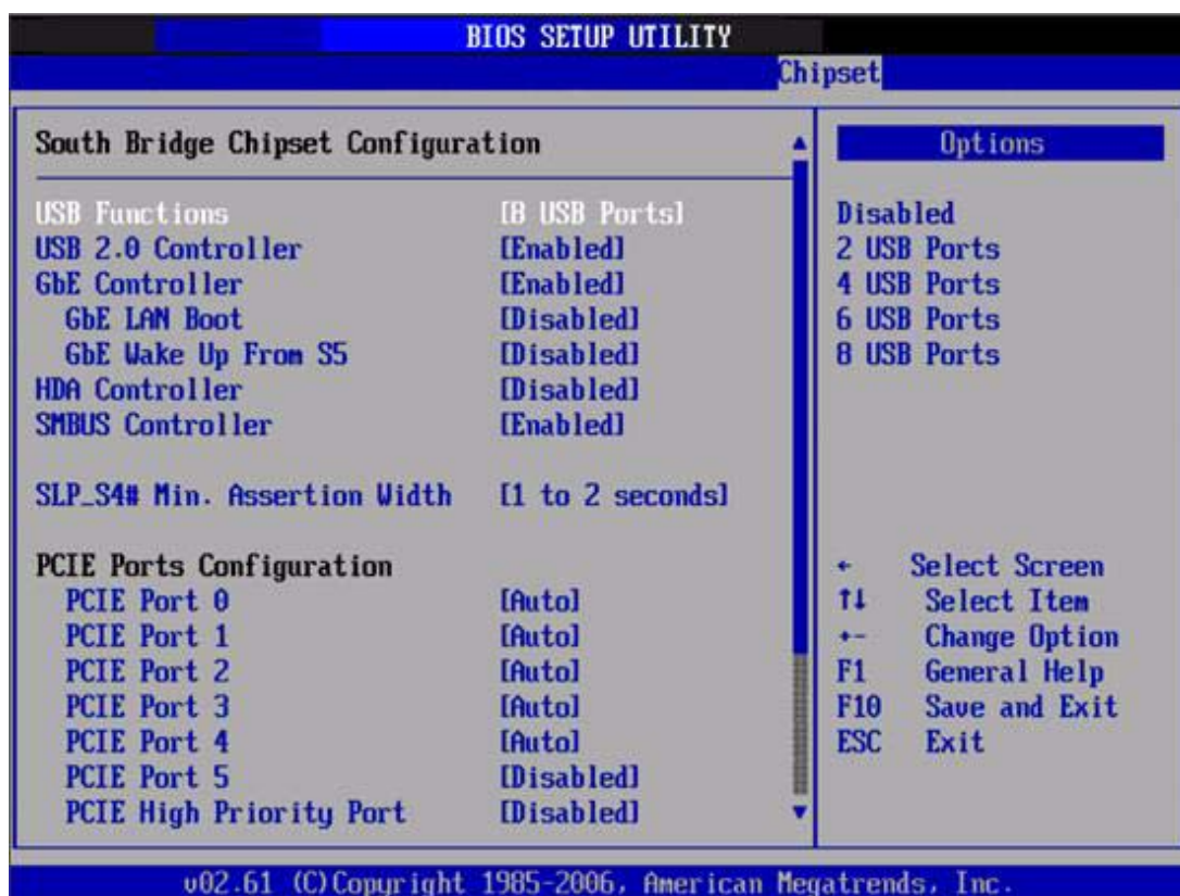
Figure 3.27 South Bridge Configuration
