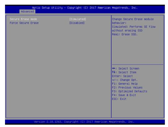
**Figure 3.12 Secure Erase Configuration**
