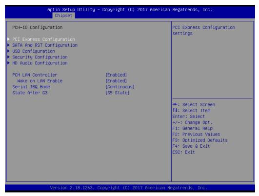
Figure 3.41 PCH-IO Configuration
