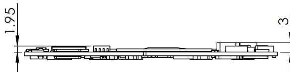
Figure 2.10 Pentium_Celeron_N_J Series Board Mechanical Diagram – Side2
