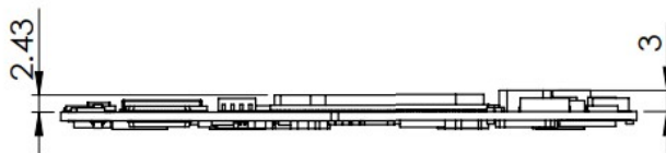
Figure 2.6 Atom_E3900 Board Mechanical Diagram - Side2
