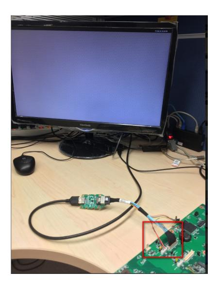
Step 3: Power on. (Please note that ROM-EG56 IC is extremely sensitive, only plug/unplug it while the DC+12V is unplugged)
