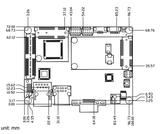
Figure 2.4 Board dimension layout (Bottom side)
