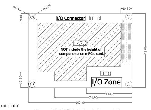
Figure 2.11 MI/O Module height constraint
