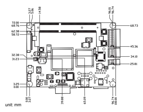
Figure 2.3 Board dimension layout (Top side)
