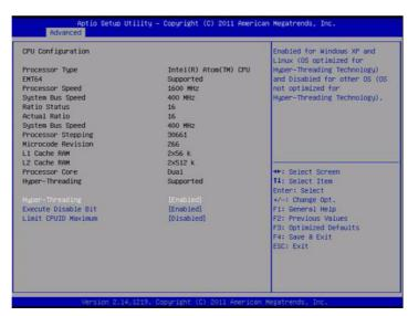
**Figure 3.6 CPU Configuration**
