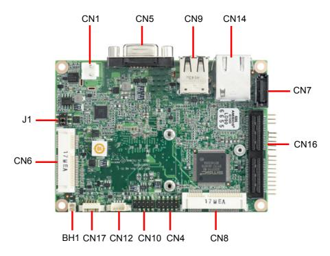
Figure 2.2 Jumper and connector layout (Bottom side)
