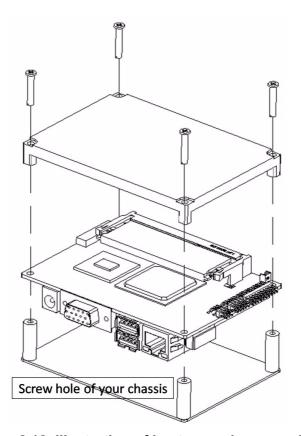
Figure 2.12 Illustration of heat spreader assembly
