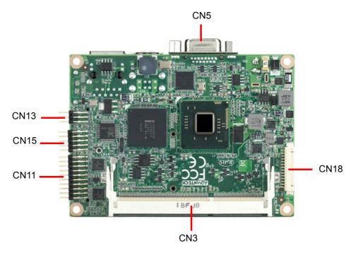
Figure 2.1 Jumper and Connector layout (Top side)
