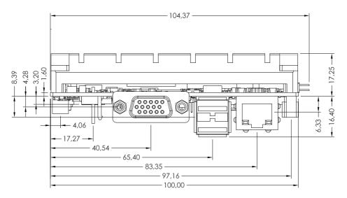
Figure 2.7 Board dimension layout (coastline with power connector and heatsink)
