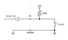
Each of the 8 isolated digital input channels accept voltages from 5 to 24 V and have a resistance of 2.0 kw. Every eight input channels share one external ground. (Channels 0~3 use EI.COM1. Channels 4~7 use EI.COM2.) The following figure shows how to connect an external input source to the card's isolated inputs:
