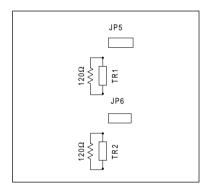
CAN termination resistor installation
