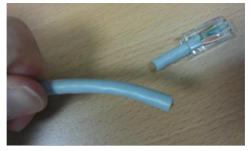
Step 3: Put all parts of RJ45 plug cable set through cable in order.
