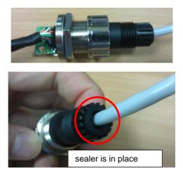
Step 8: Press the cable hard inward and lock the plastic rear nut tightly at the same time.
