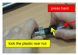
Step 9: Tighten the plastic rear nut more to make sure the cable is secured from being moved by any unexpected force.
