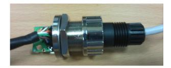
Step 7: Screw on the plastic rear nut a little bit for later locking. Make sure sealer is in place.
