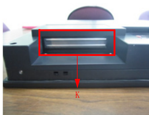
Figure 2.5 PCI expansion slot
