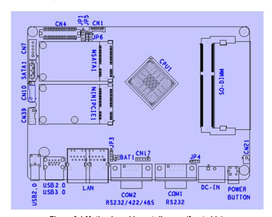
Figure 3.1 Mother board layout diagram (front side)
