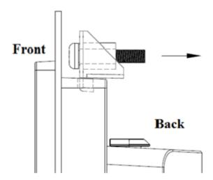
Figure 2.29 Hooks bracket location
