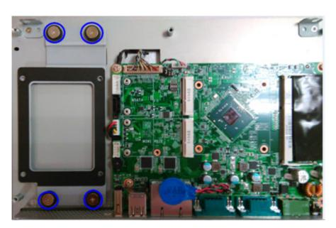
Figure 2.8 Retention screw on HDD bracket
