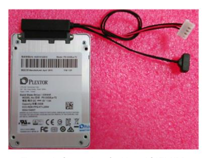
Figure 2.10 Connection of cable and SATA HDD
