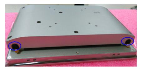
Figure 2.19 Remove plugs for antenna
