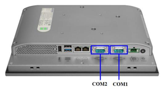
Figure 3.2 COM1 and COM2 Position
