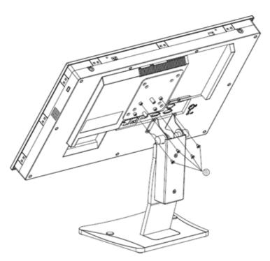
Figure 2.35 Securing VESA Bracket
