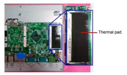
Figure 2.7 Attach thermal pad on memory
