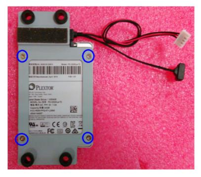
Figure 2.11 Secure SATA HDD with screws
