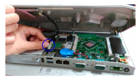
Figure 2.20 Reinstall the rear cover
