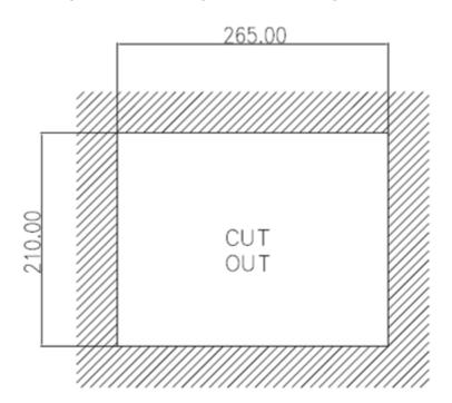
Figure 2.26 PPC-3100S Cut-out dimension
