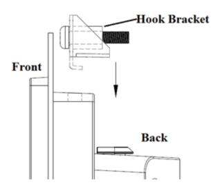
Figure 2.28 Hooks bracket for panel mounting
