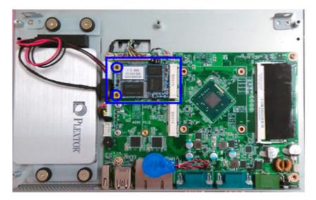
Figure 2.13 Install mSATA module
