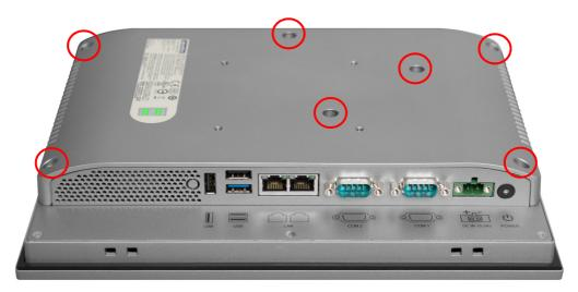
Figure 2.4 Retention screw on rear cover
