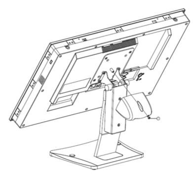
Figure 2.36 Securing Hinge Cover
