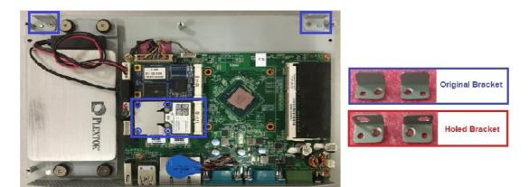
Figure 2.14 Install wireless LAN card
