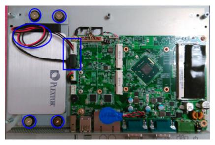
Figure 2.12 Connect SATA HDD to Mainboard
