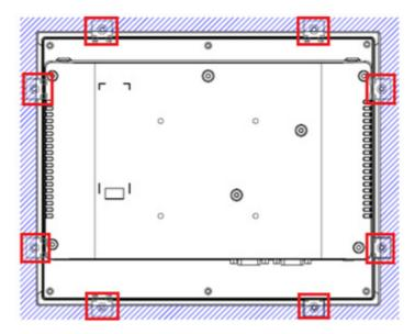
Figure 2.31 Back side view of panel mounting
