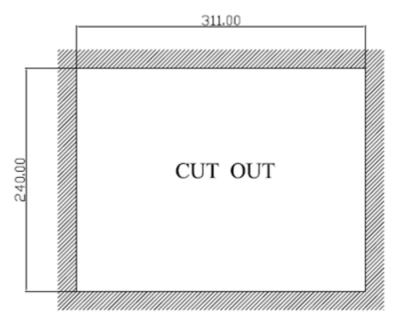
Figure 2.27 PPC-3120S Cut-out dimension
