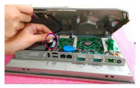
Figure 2.5 Remove cable from Mainboard
