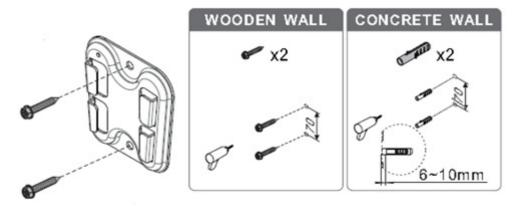
Figure 2.22 Mounting bracket on the wall
