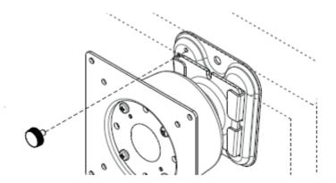
Figure 2.25 Secure the Panel PC
