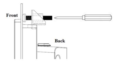
Figure 2.30 Fasten the Hook bracket
