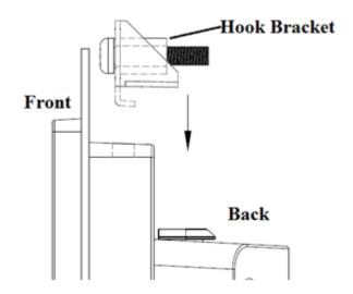
Figure 2.25 Hook Brackets for Panel Mounting
