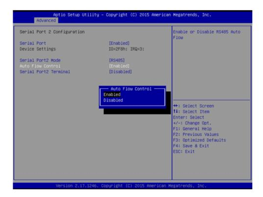
5. When COM2 Mode is selecting RS485, "Serial Port2 Terminal" also can select [Enabled] or [Disabled]
