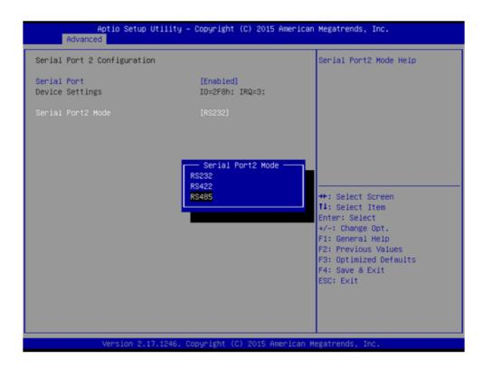
4. When COM2 Mode is selecting RS485, "Auto Flow Control" also can select [Enabled] or [Disabled]
