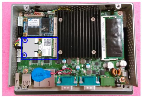
Figure 2.15 Install Full-size Wireless LAN Card
