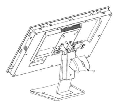
Figure 2.33 Securing the Hinge Cover
