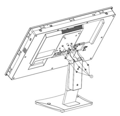
Figure 2.32 Securing VESA Bracket
