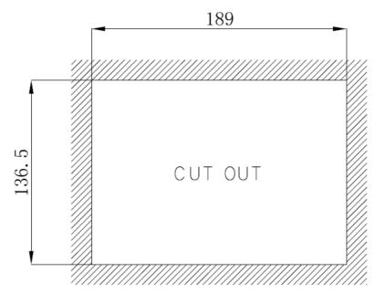
Figure 2.24 PPC-3060S Cut-out Dimensions
