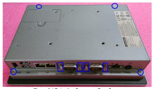
Figure 2.4 Retention Screws on Rear Cover
