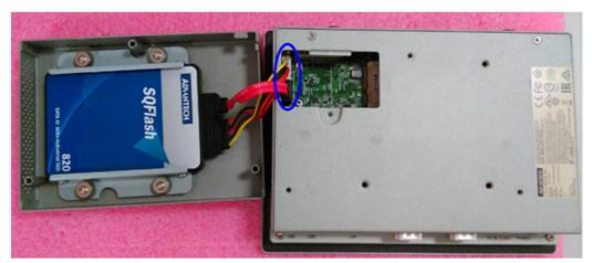
Figure 2.12 Connecting the SATA HDD to the Mainboard
