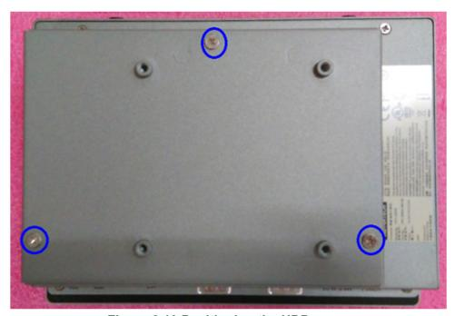
Figure 2.13 Positioning the HDD cover
