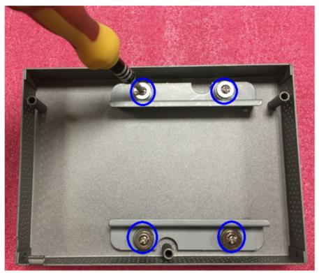
Figure 2.7 Retention Screws on the HDD Bracket
