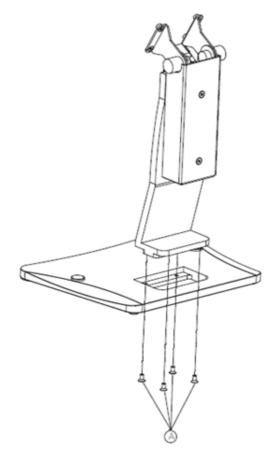
Figure 2.31 Securing the Base
