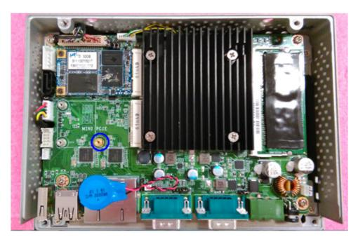
Figure 2.16 Location of Retention Screws
