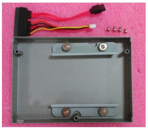
Figure 2.8 HDD Module
