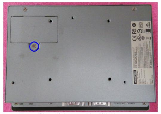
Figure 2.11 Removing the mSATA Door
