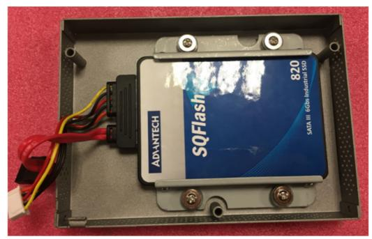
Figure 2.10 Installing the HDD into the HDD cover
