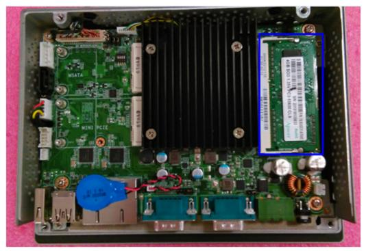
Figure 2.5 Installation of Memory Card
