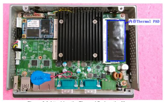
Figure 2.6 Attaching the Thermal Pad on the Memory
