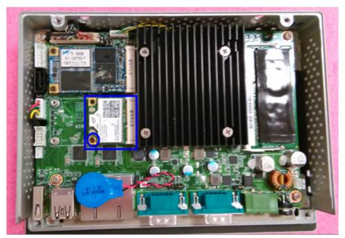
Figure 2.17 Install Half-size Wireless LAN Card
