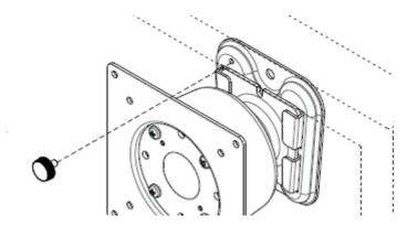
Figure 2.23 Secure the Panel PC
