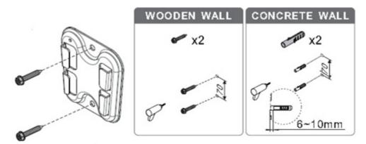
Figure 2.20 Mounting the Bracket on the Wall
