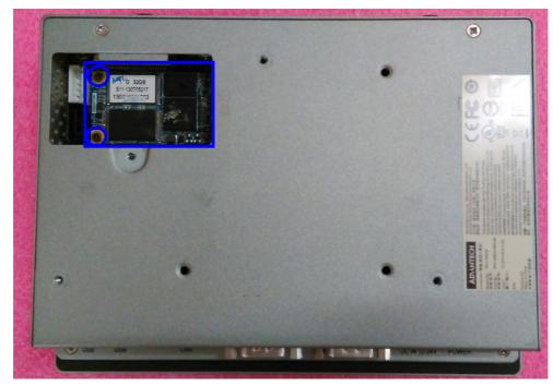
Figure 2.14 Installing the mSATA Module
