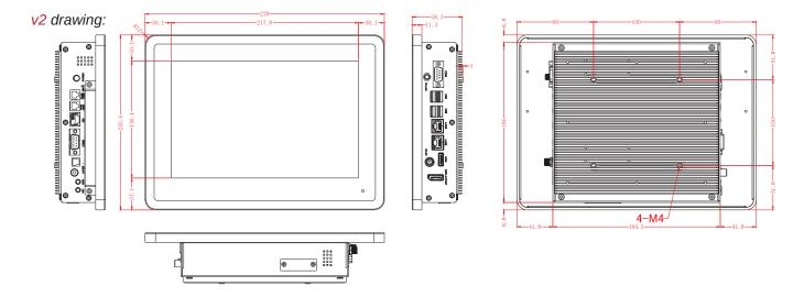
Added screwholes for the the clamp support mounting option
