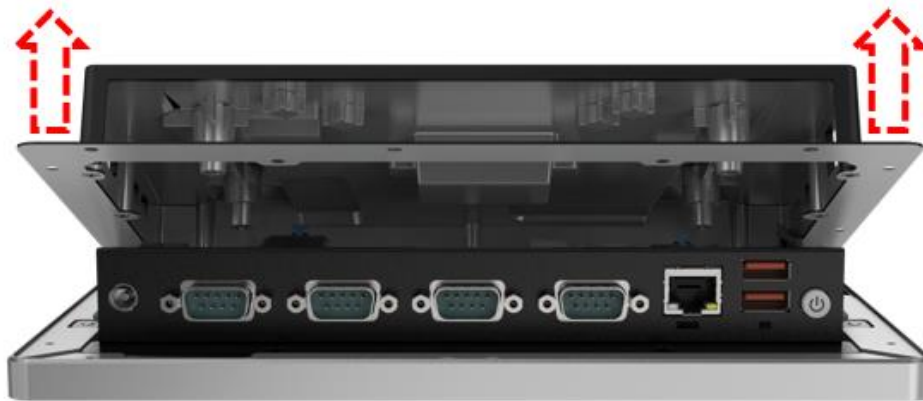
Figure 3-2: Remove the Back Cover
