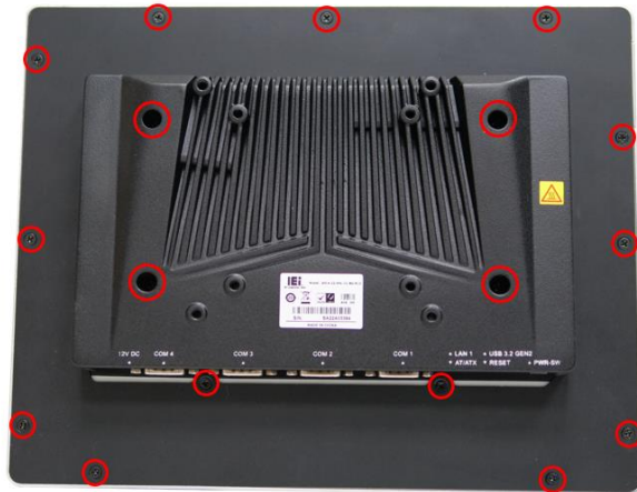
Figure 3-1: Back Cover Retention Screws
