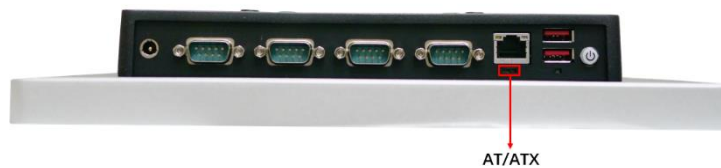
Figure 3-6: AT/ATX Switch Location
