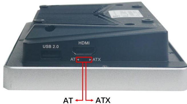
Figure 3-5: AT/ATX Switch Location
