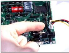
On SOM-100ES carrier revisions prior to revision 5, the power supply jumper (JP3) must be set according to the type of power supply. Revision 5 boards have no jumper setting requirements related to the type of power supply so skip to the next section if you have a revision 5 board.
