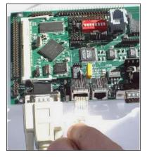
A network connection may be established by connecting the carriers Ethernet jack to a standard 10/100 base-T network.
