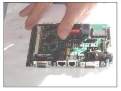
Insert the SoM into the SODIMM socket of the SoM-100ES.
