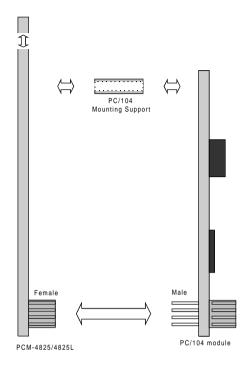
Figure B-1: PC/104 module mounting diagram
