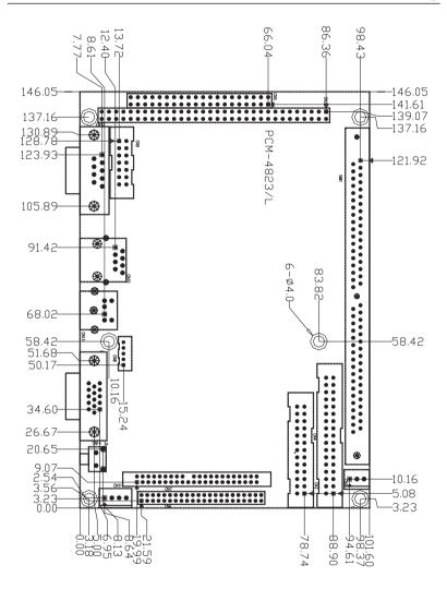
Figure E-1: PCM-4823/4823L Mechanical Drawing
