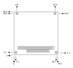
Figure B-2: PC/104 module dimensions (mm) (±0.1)
