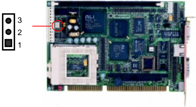
CPU fan power connector (CN4)
