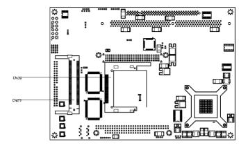
Figure 2.2: Jumper & Connector (solder side)
