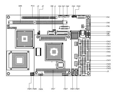
Figure 2.1: Jumper & Connector (component side)
