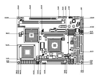
Figure E.1: PCM-9582 Mechanical Drawing (component side)
