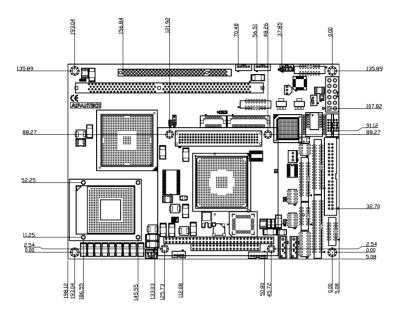
Figure 1.1: Board layout: dimensions (component side)
