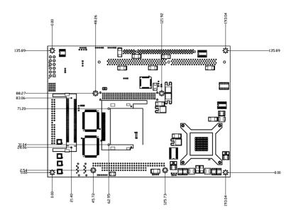
Figure 1.2: Board layout: dimensions (solder side)
