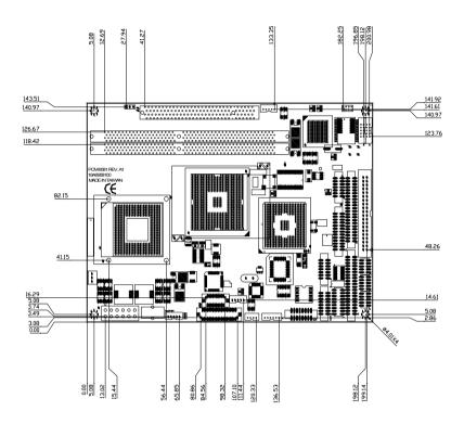
Figure 1.1: Board layout: dimensions (component side)
