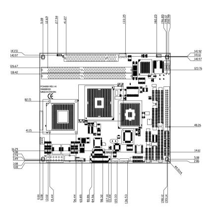
Figure E.1: PCM-9581 Mechanical Drawing (component side)
