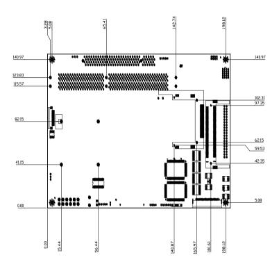
Figure E.2: PCM-9581 Mechanical Drawing (solder side)
