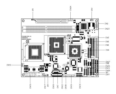
Figure 2.1: Jumper & Connector (component side)
