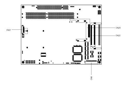
Figure 2.2: Jumper & Connector (solder side)
