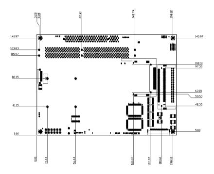
Figure 1.2: Board layout: dimensions (solder side)
