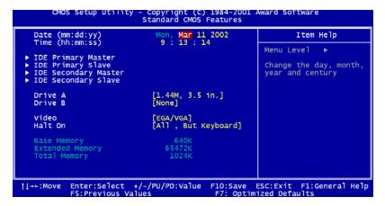
Figure 4.2: CMOS Features setup
