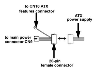
Figure 2.3: Wiring for ATX soft power switch function
