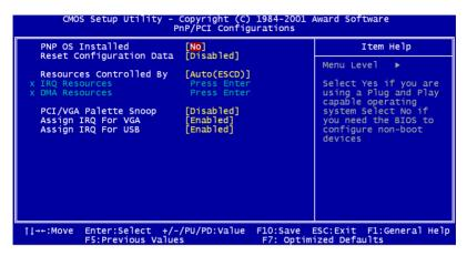
Figure 3.7: PnP/PCI Configurations
