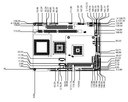
Figure F.1: PCM-9577 Mechanical Drawing (component side)
