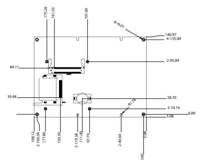
Figure F.2: PCM-9577 Mechanical Drawing (solder side)
