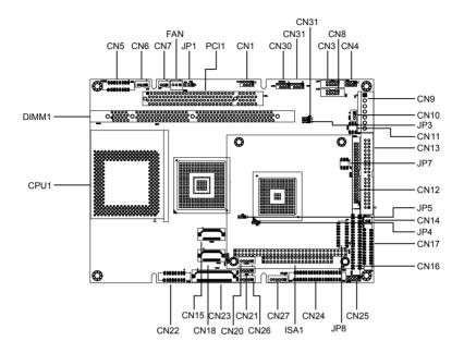
Figure 2.2: Connectors (component side)
