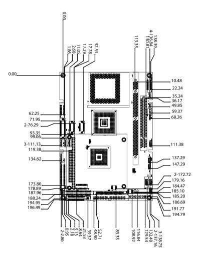
Figure 1.1: Board layout: dimensions
