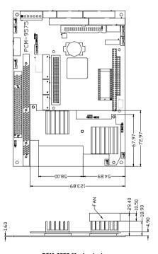
PCM-9575 Mechanical (Side view for PCM-9575F-Q0A1 only)
