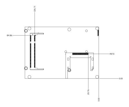
Figure 1.2: Board layout: Dimensions(Solder Side)
