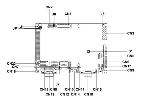
Figure 2.1: Jumpers and Connectors Drawing (component side)
