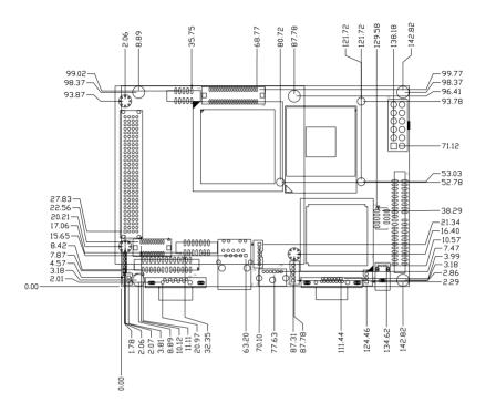
Figure 1.1: Board layout: Dimensions(Component Side)
