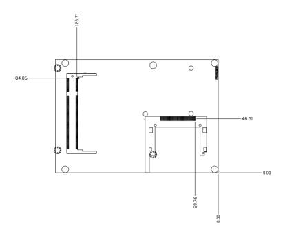
Figure F.2: PCM-9381 Mech Drawing (Solder Side)
