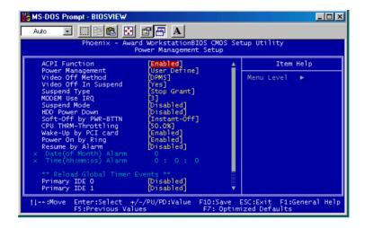
Figure 4.5: Power management setup screen
