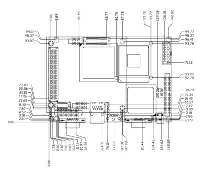
Figure F.1: PCM-9381 Mech Drawing(Component)
