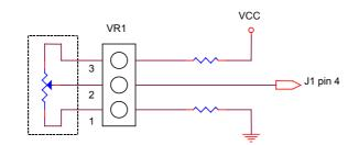
Variable Resistor (Recommended: 4.7KΩ, >1/16W)
