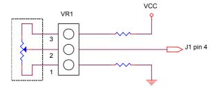
Variable Resistor (Recommended: 4.7KΩ, >1/16W)
