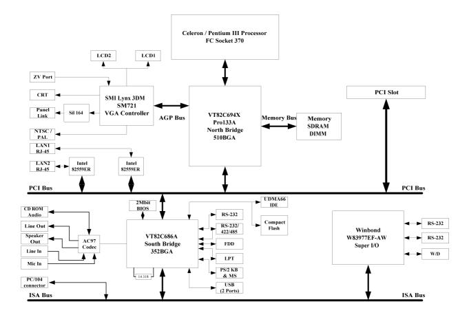
The two key components on board are the VIA VT82C694X North Bridge and VT82C686A super South Bridge. These two devices provide the ISA and PCI bus to which all the major components are attached.
