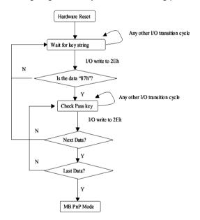
There are three steps to complete the configuration setup: (1) Enter the MB PnP Mode; (2) Modify the data of configuration registers; (3) Exit the MB PnP Mode. Undesired result may occur if the MB PnP Mode is not exited normally.
