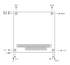
Figure C-2: PC/104 module dimensions (mm) (±0.1)
