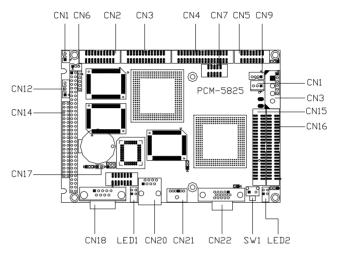
Figure 2-2: Connectors - component side
