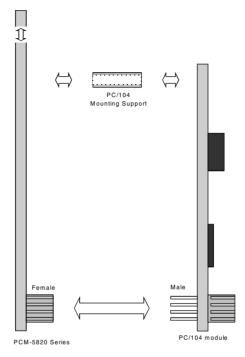
Figure C-1: PC/104 module mounting diagram
