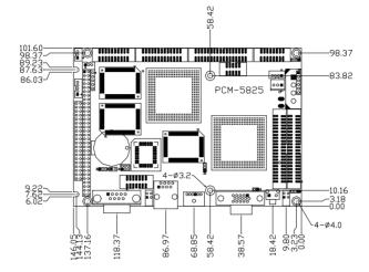
Figure E-1: Board Dimensions component side
