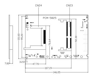
Figure E-2: Board Dimensions solder side
