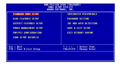
Figure 4-1: BIOS setup program initial screen
