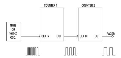
The Intel 8254 has six operational modes, from Mode 0 through Mode 5. To generate a pacer clock, program both Counter 1 and Counter 2 for Mode 3 (square wave generation).
