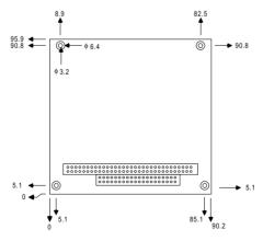
Figure B-2: PC/104 module dimensions (mm) (±0.1)
