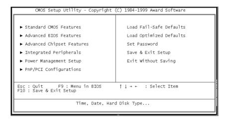
Figure 4-1: BIOS setup program initial screen
