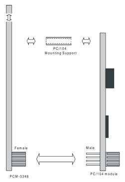
Figure B-1: PC/104 module mounting diagram
