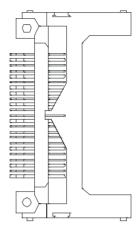
Figure C-1: CompactFlash™ socket
