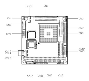
Figure 2.1: Locating connectors (component side)
