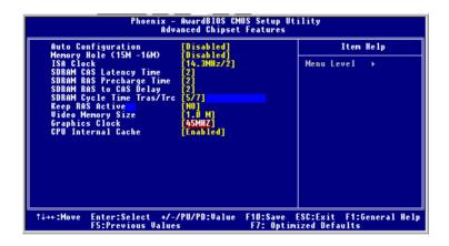
Figure 4.3: Advanced chipset setup
