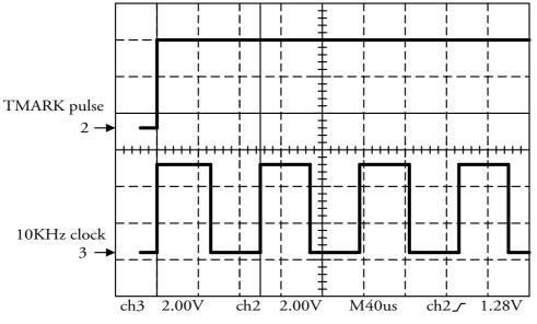
Figure 2. 10KHz Clock/UTC TMARK Pulse Relationship
