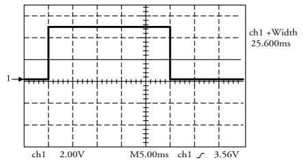
Figure 1. GPS Receiver Time Mark Pulse Waveform.
