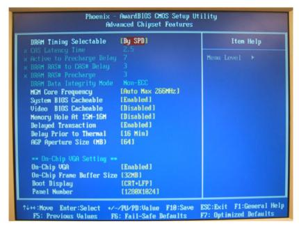
Figure 4.4: Advanced Chipset Features setup
