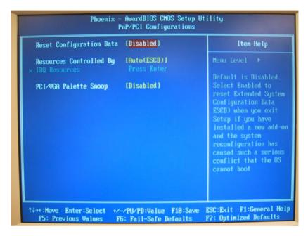
Figure 4.7: PnP/PCI Configurations
