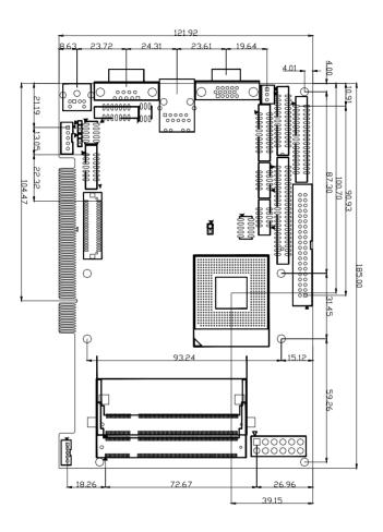
Figure 1.1: Board layout: dimensions (component side)
