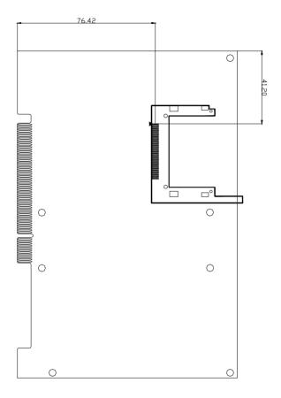
Figure 1.2: Board layout: dimensions (solder side)
