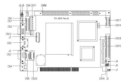
Figure 2.1: Jumper & Connector location (component side)
