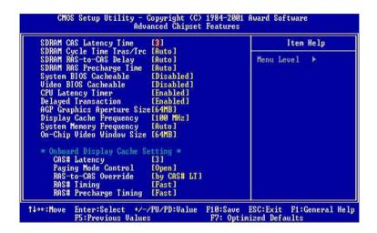
Figure 3.4: Advanced Chipset Features screen
