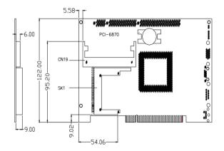
Figure 1.2: PCI-6870 dimension (solder side)
