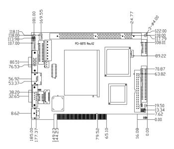
Figure 1.1: PCI-6870 dimension (component side)
