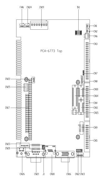
Figure 2.1: Jumper & Connector locations
