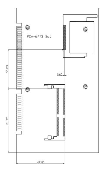
Figure 1.2: Board layout: dimensions (solder side)
