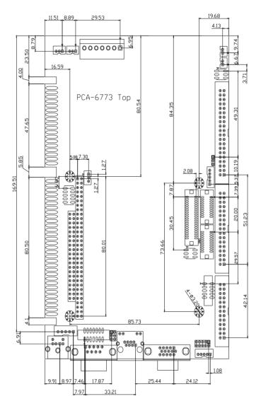
Figure 1.1: Board layout: dimensions (component side)
