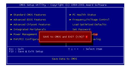
Figure 4.12: Save to CMOS and EXIT
