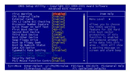
Figure 4.3: Advanced BIOS Features setup
