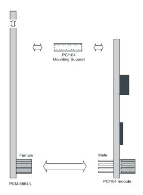
Figure B.1: PC/104 module mounting diagram
