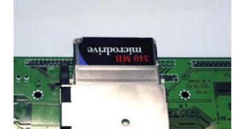
Step 1: Plug in CompactFlash Card
