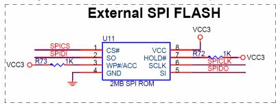
If pin 3 (WP#) in above circuit is pulled high, SPITool can accept "protect" and "unprotect" parameters to set write protection of SPI flash disk. After you setup SPI flash disk and disable changing write protection mode of flash disk, please connect pin 3 to low.
