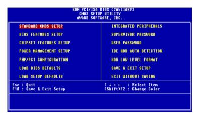
Award's BIOS ROM has a built-in Setup program that allows users to modify the basic system configuration. This type of information is stored in battery-backed CMOS RAM so that it retains the Setup information when the power is turned off.
