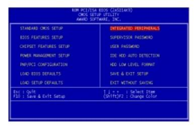
Integrated Peripherals options are displayed by choosing the INTEGRATED PERIPHERALS icon from the INITIAL SETUP SCREEN. This section sets the IDE transfer mode for all IDE channels. It also configures the other onboard ports. The following configurations are based on the manufacturer's SETUP DEFAULTS settings.
