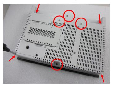
Step 2: Unfasten the screws on the HDD bracket
