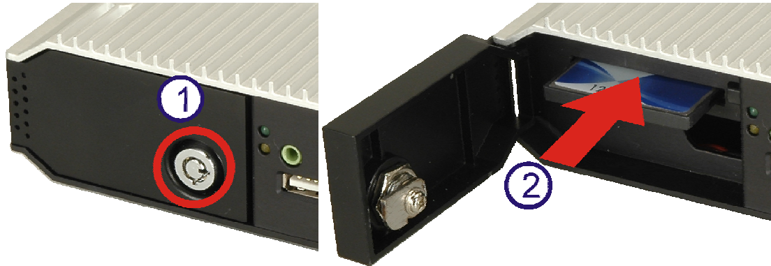
Figure 4-1: CompactFlash® Card Installation
