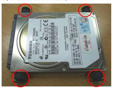
Step 4: Put the 2.5" SATA onto HDD bracket
