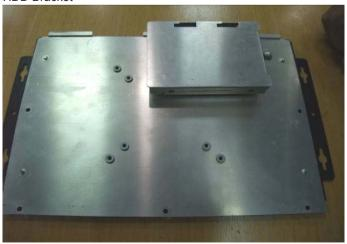
Step 3: Fasten four screws with the dampers on the 2.5" SATA HDD
