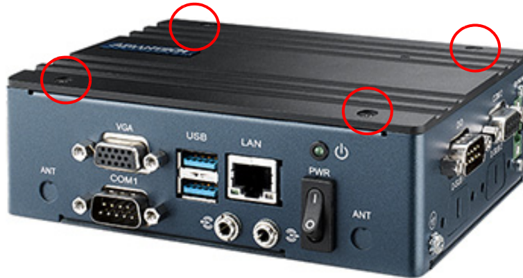
Figure 2.15 Loosen Screws, Open TOP Case
