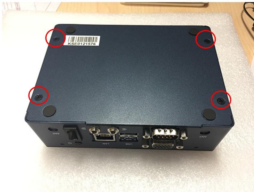
Figure 2.17 Loosen Screws, Open Bottom Case
