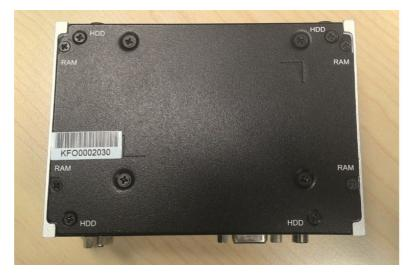
2. Remove the four snap rivets from the bottom cover.
