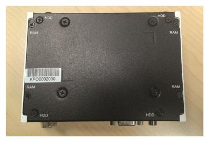
2. Unscrew the four screws on the sides of ARK-1123.
