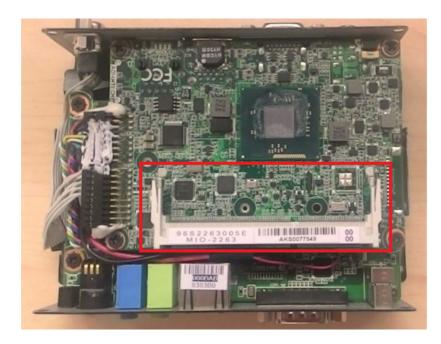
5. Replace the aluminum top chassis and secure all screws.
