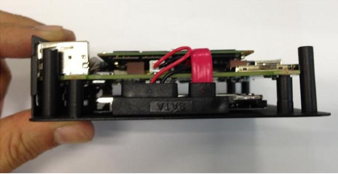
11. Use the screws included with EBOX to secure the HDD.
