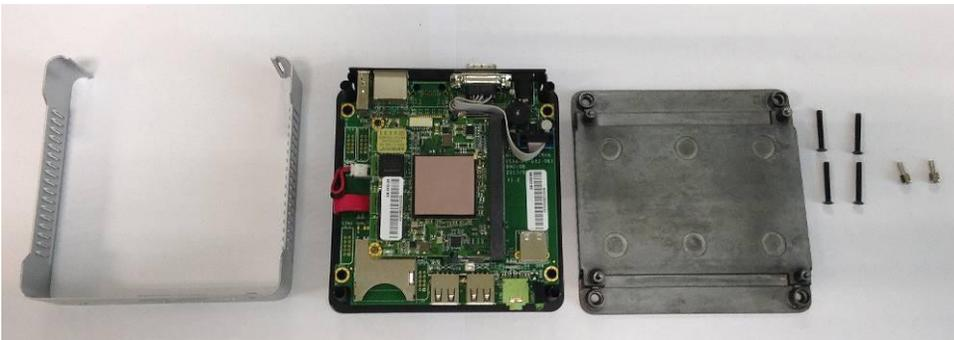
7. Remove the board, can keep the power line connected.
