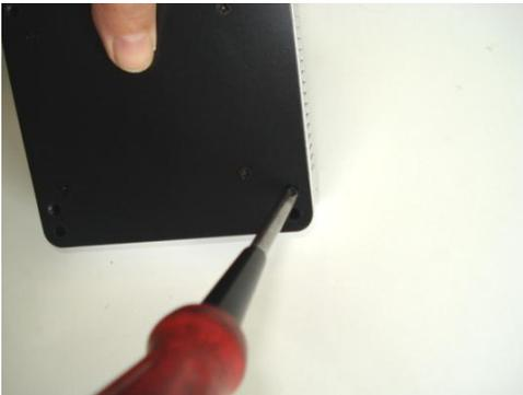
3. Remove two screws next to the VGA port at rear side.
