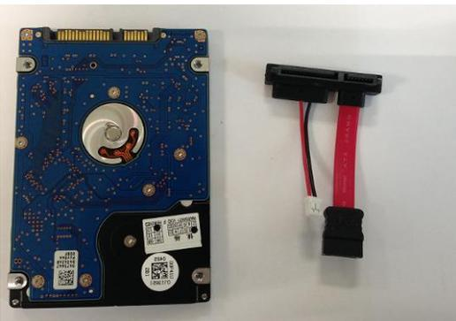
9. Connect the cable to the HDD connector.
